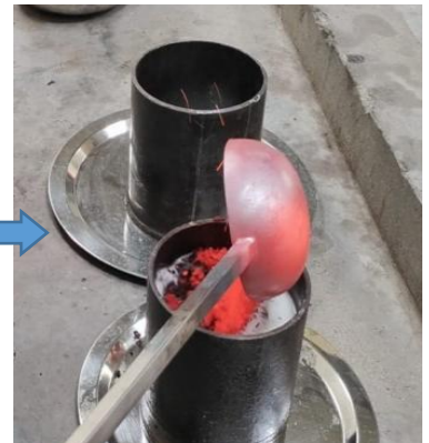
Quenching in Takra
