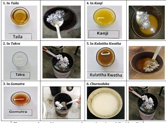
The process of quenching was repeated seven times in each liquid media
