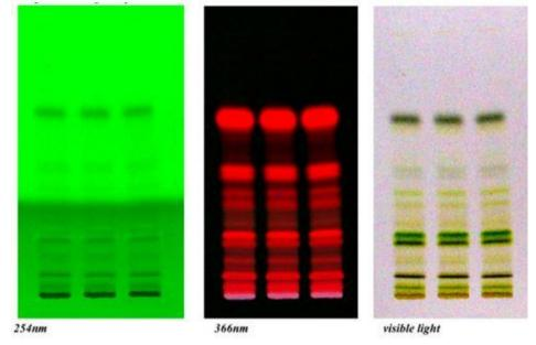
Figure 9: HPTLC plate visualized under (a) UV 254 nm (b) UV 366 nm (C) White light
